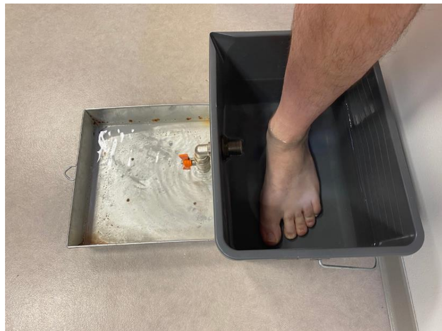
Figure 2. A volumeter was set up with a tap allowing overflow. After filling above the level of the tap, the latter was opened to obtain the reference level (after a few minutes in order to obtain flat, stable water). The feet of the subjects were slowly immersed until both feet stood firmly on the ground, causing the displacement of a volume of liquid outside the volumeter through the tap. The liquid corresponding to the volume of the submerged foot was then collected and weighed.
